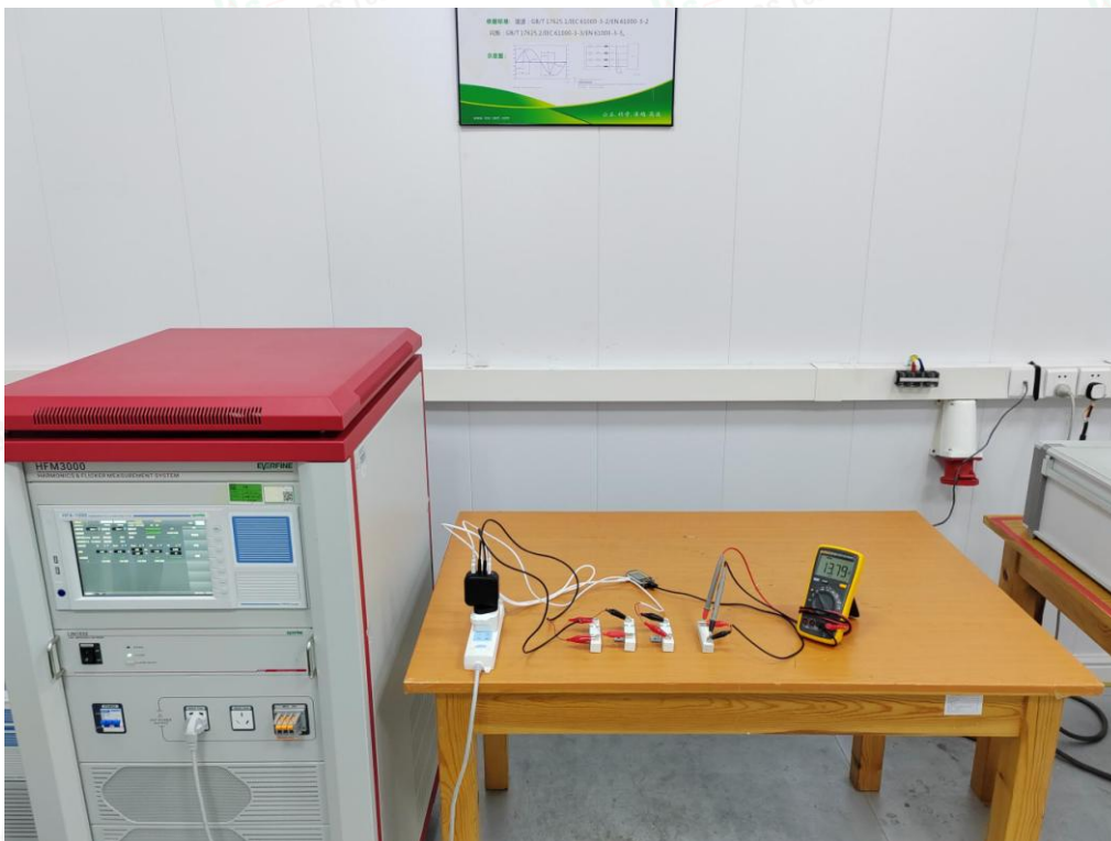
Test Setup Photo of Harmonic & Flicker Measurement
